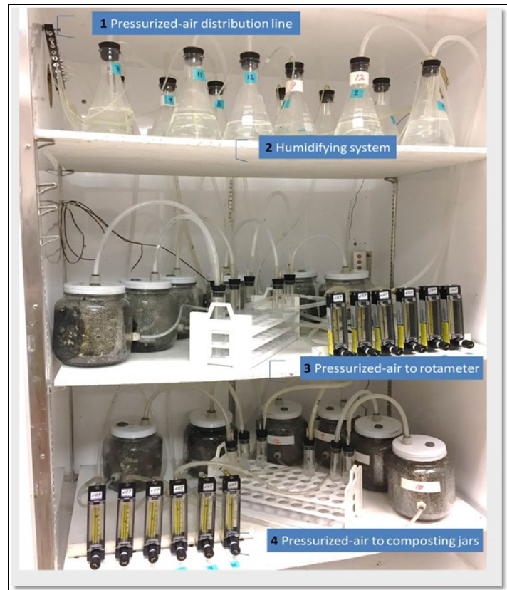
Figure 3. Laboratory apparatus employed to measure the biodegradability of plastic mulches under composting conditions via the ASTM D5338 standardized laboratory test.
