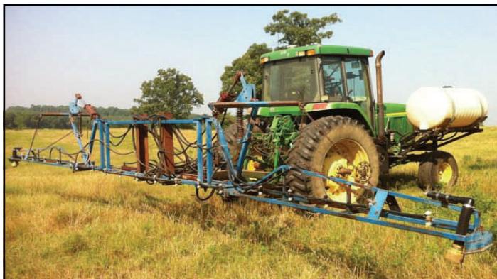
Fig. 2. Herbicide applications made on calm days with low pressures and low boom heights can reduce the likelihood of physical drift.
