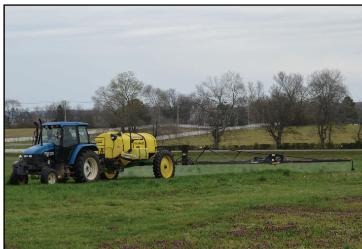
Fig. 2. Herbicide applications made on calm days with low pressures and low boom heights can reduce the likelihood of physical drift.
