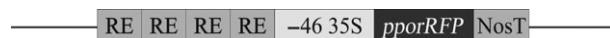
Figure 1 Synthetic promoter design [adapted from Liu et al. (2011)]. Tetramer of regulatory element sequence was placed upstream of the minimal CaMV 35S (i.e. -46 35S) promoter and orange fluorescent protein reporter ( pporRFP ) from Porites porites (Alieva et al. , 2008).
