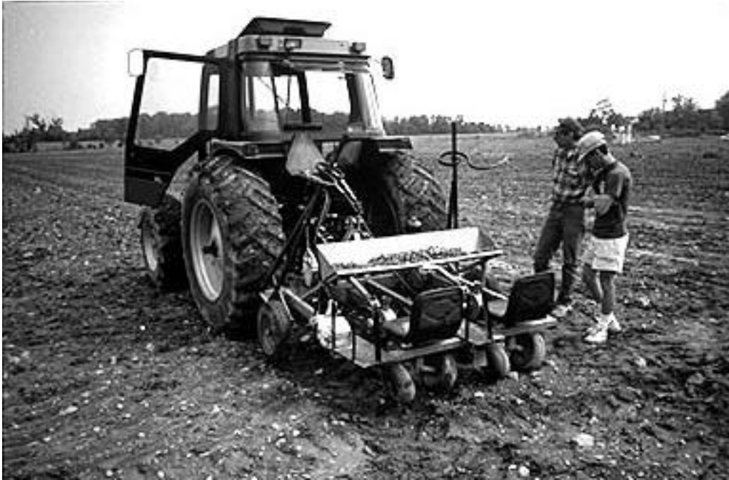
Figure 2. The Fröbbesta planter uses 25cm long cuttings as planting stock and plants one double row at a time.
