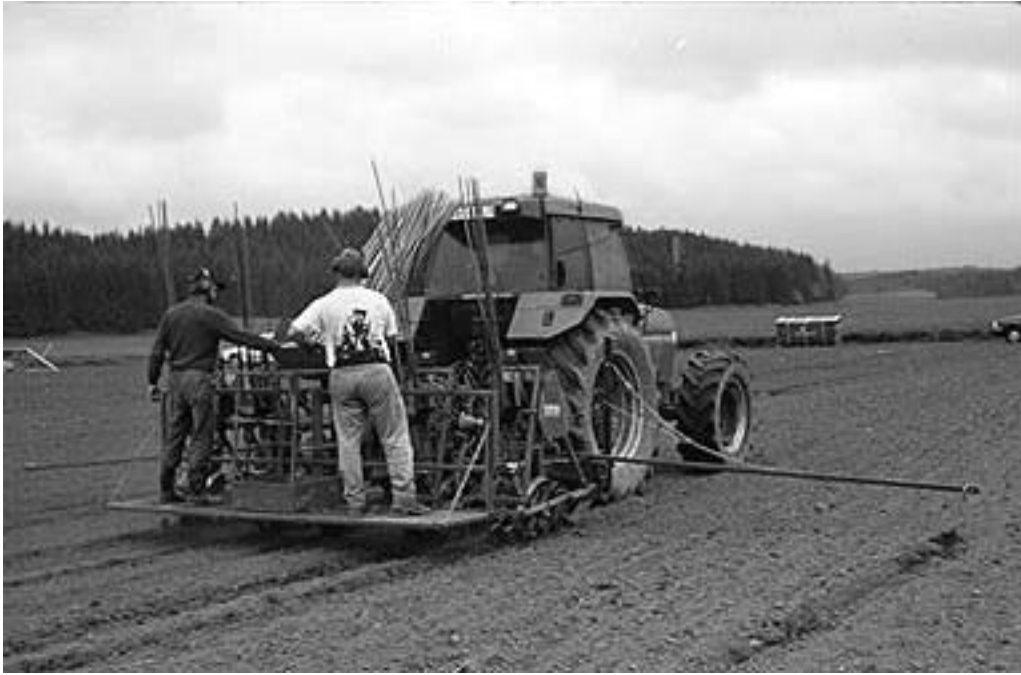
Figure 3. The Step planter uses 1 – 2 m whips as planting stock and plants two double rows at once.
