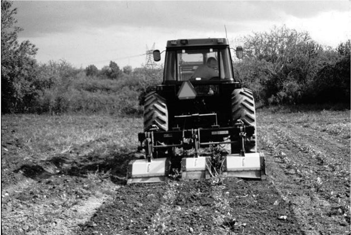
Figure 4: The Badalini tractor mounted rototiller is used to control weeds in willow biomass crops. Individual heads are spaced to fit the double row spacing. This willow crop is early in its first year of growth following coppice.
